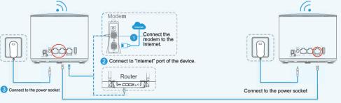
Connect the cable to LAN port of one mesh device.
